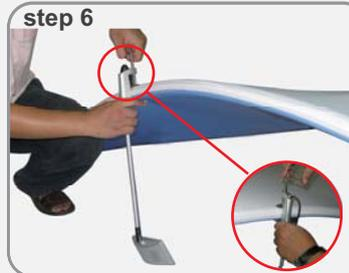
Hand-tight the LED light (E) on the top of frame, and connect with the power cord.
